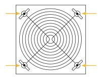
Unpack the custom carbon filters and remove the four wing nuts on the back side of the fan, then remove the fan grill from the fan.
