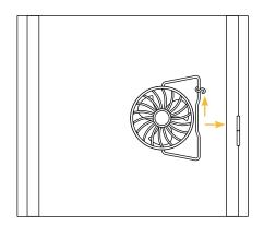
Locate the internal circulation fan. Note the "S" hook connected to the base of the fan. This hook will fit into the notches located on the backside of the inner door frame. Mount the Fan on one of the lower notches. As the plants grow taller, move the fan to the upper notches. Ideally the fan will blow air across the top of the plants. Thread cord through the upper hole found on the lower interior of the cabinet (same as the light power cord).
