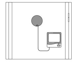
Locate the thermometer/hygrometer. Remove the battery cover and remove the plastic safety blocker from the battery terminal. Use the included velcro strips to affix your thermometer/hygrometer to the inside of your cabinet. The best placement for this is towards the top of the cabinet, either on the side or back wall.
