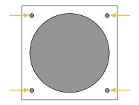
Locate the large opening in the back of the cabinet with the four small surrounding holes. With the help of a partner hold the carbon filter and fan flush to the inside back of the cabinet. Make sure to place the four bolts through the four provided holes. The power cord remains inside the cabinet **NOT THROUGH THE FAN HOLE OPENING.**
