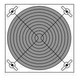
Have a partner place the fan grill on the outside of the cabinet on the four filter fan bolts, then tighten the wing nuts onto the exposed bolts. Repeat the previous steps for the other carbon filter/fan.
