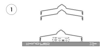
Unpack the KIND LED Grow Light and locate the wire hangers. Connect the wire hangers to each of the metal hangers on the light.
