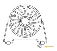
Locate the internal circulation fan. Note the "S" hook connected to the base of the fan. This hook will fit into one of the two provided notches located on the backside of the inner door frame.
