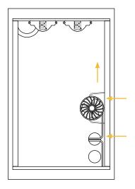
Mount the fan on the lower notch. As your plants grow taller, move the fan to the upper notch. Ideally the fan will blow air across the top of the plants. Thread the power cord through the upper hole found on the lower interior of the cabinet (same as the carbon filter cord).
