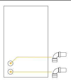
From the outside of the cabinet, insert the foam side of the two 2 in. elbows into holes located at the bottom corner in rear of the cabinet. Be sure to adjust the elbows so the openings face towards the center of the cabinet
