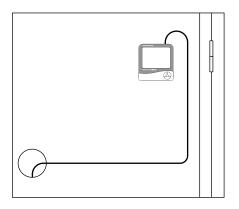
Locate the thermometer/hygrometer. Remove the battery cover and remove the plastic safety blocker from the battery terminal. Use the included velcro strips to affix your thermometer/hygrometer to the inside of your cabinet. The best placement for this is towards the top of the cabinet, either on the side or back wall.
