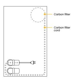
Locate the power cord for the carbon filter and thread the cord through the upper hole found on the lower interior of the cabinet.
