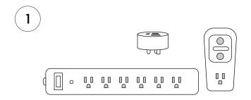
Locate the power strip, the GFCI protector, the smart plug, and the 3-IN-1 adapter.
